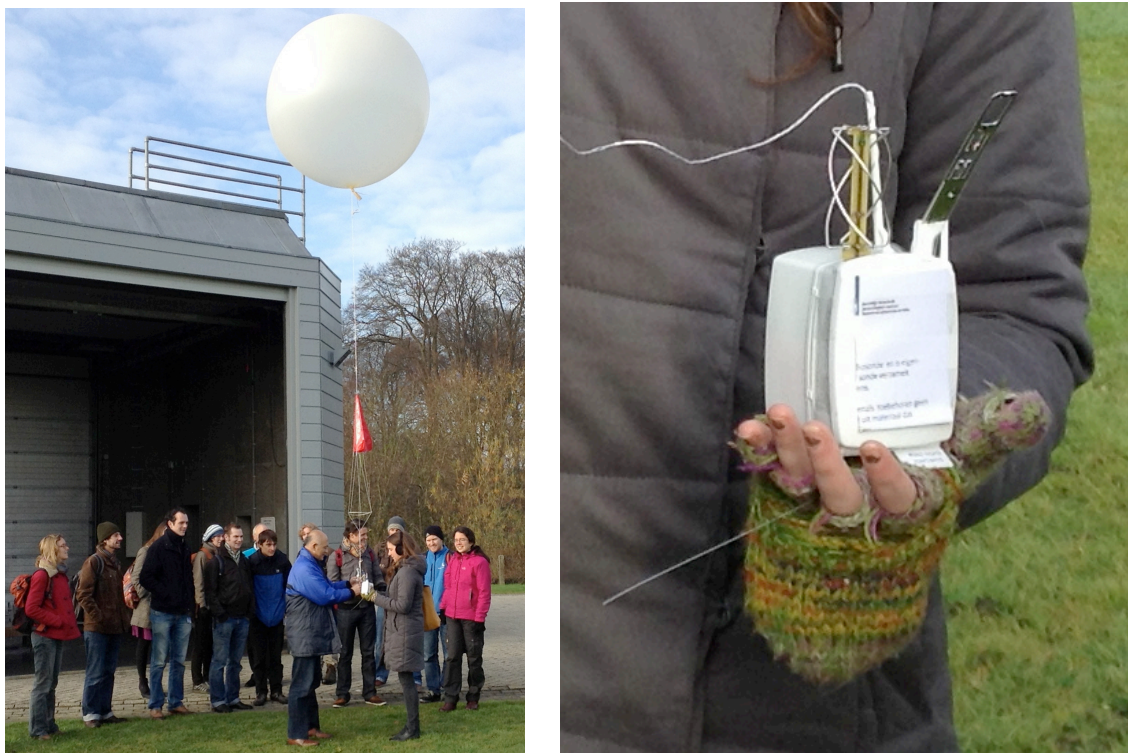
Figure 0.1: Launching a radiosonde with Climate Physics master students on 30 November 2012 during an excursion to the Dutch National Weather Service (KNMI) A balloon filled with helium (picture at left) carries an instrument (picture at right) that measures pressure, temperature and humidity up to a height of about 20 to 30 km above sea level. During its ascent to a height of 20 to 30 km above sea level, the balloon is tracked by radar. The wind-vector as a function of pressure is determined from the position of the balloon.
